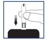
1 Insert the test strip to turn on the monitor.
