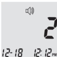
To turn off the voice press and release the bottom button until 0 appears. Press and release the middle button to set VOICE FEATURE OFF. The meter will now beep instead of speaking. To turn the voice feature on if turned off follow steps 1-3.
