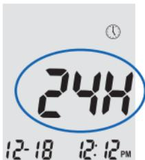
**Step 7: Set Hour:** The current hour will flash. If the talking feature is on, the meter will say, “Set Hour.” Press the up or bottom button to reach the correct hour.
