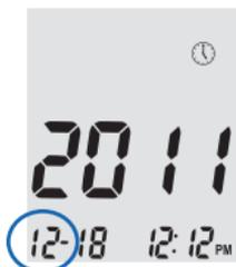
**Step 5: Set Day:** The current date will flash. If the talking feature is on the meter will say “Set Day”. Press and release the up or down button to reach the desired day. When the desired day is reached press and release the middle button.
