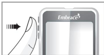
**Step 2:** Press and release the middle button to enter the set up screen. Then press and release the up or down button until the
