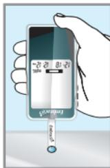
After 6 seconds the Control Solution reading will be displayed on the display screen.
